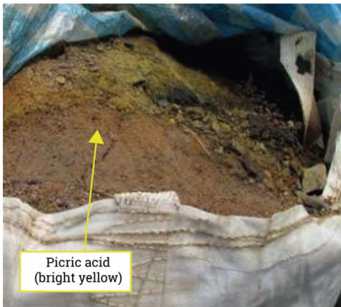
Soil contaminated with picric acid stored in bags before MuniRem treatment
