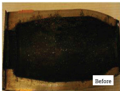
Rapid decontamination of halved bomb casings before and after MuniRem treatment
