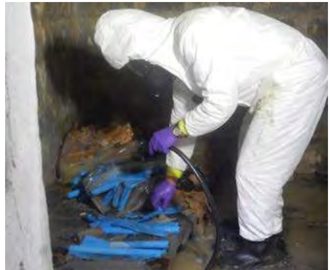
MuniRem UXO technician sprays MuniRem Solution on aged dynamite, weeping Nitroglycerin to render it safe to handle.
