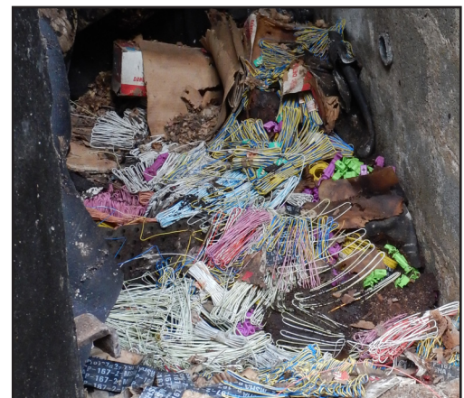
Deteriorated electric and non-electric detonators and system components safely removed and destroyed
