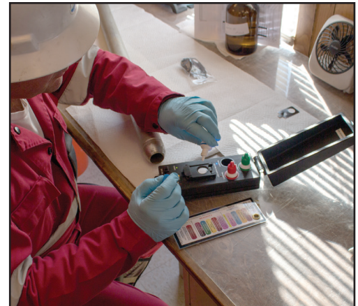
Field explosive detection kits are used to distinguish the type of explosive present
