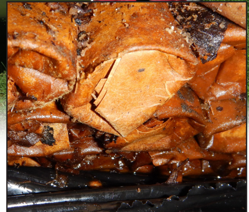
Deteriorated dynamite and visible nitroglycerin rendered safe using environmentally safe neutralization process
